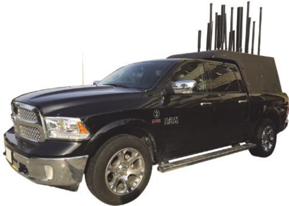
The BEAST is a wideband jamming system to protect against RCIED ( remote controlled improvised explosive devices ).
